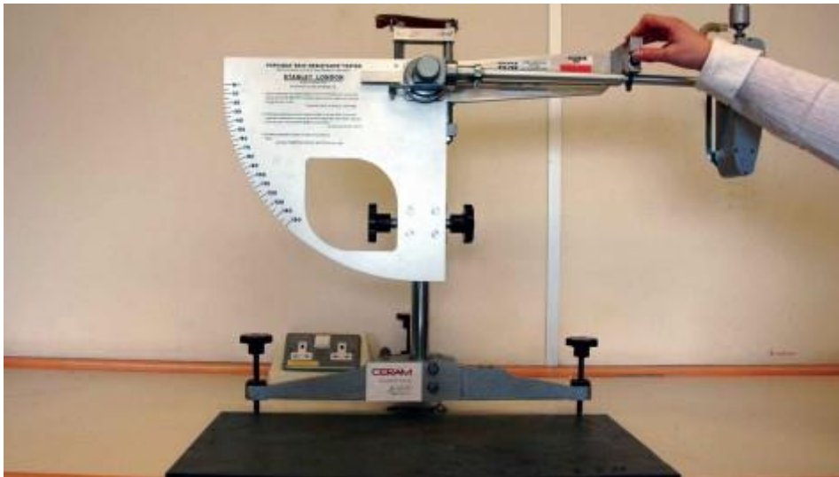
Figure 6.1 - Pendulum Test Rig
