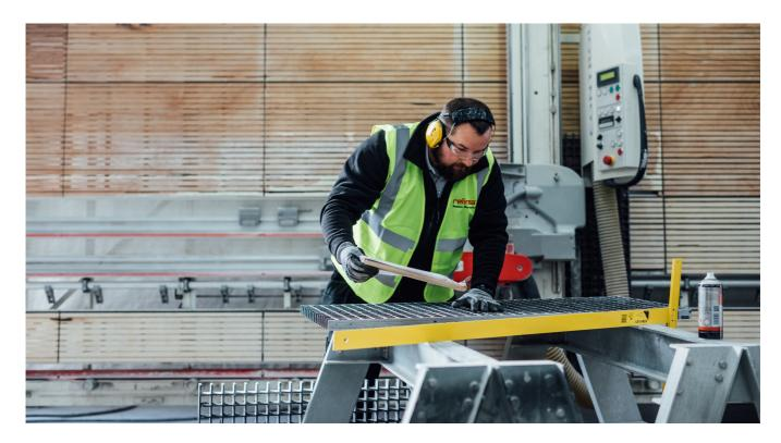
A major advantage of using Relinea's Glass Reinforced Plastic (GRP) products is the ease of fabrication — sawing, grinding, drilling and machining is similar to working with wood, metals and plastics. If possible, perform fabrication "on-site" to increase accuracy. Be sure to allow for blade width (usually 5mm) when performing take-offs and layouts. For a nice looking installation, cut panels so bars of adjoining panels are aligned and leave a solid bar on all sides
